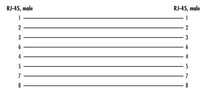
Figure 15. Typical Ethernet straight-through cable diagram for 1000Base-T
